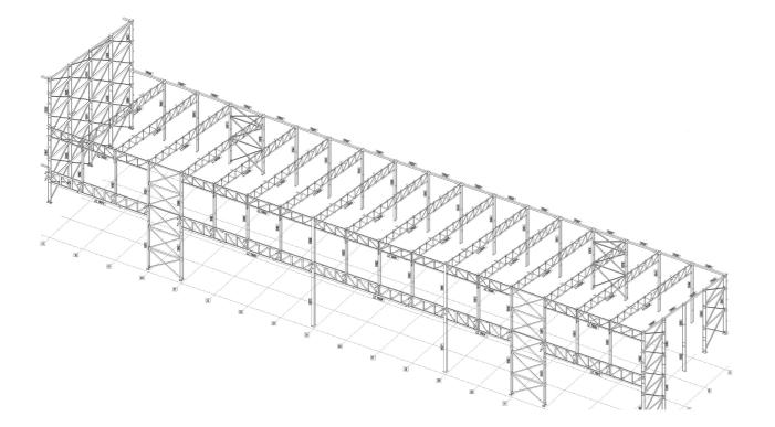
supporting structure of these buildings, with a total weight of 1.680 tons.
